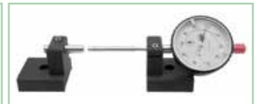
Controllo comparatori. Control of dial gauges.
