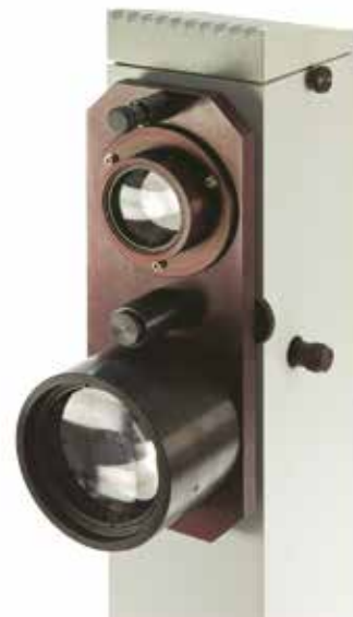
Luca per profilo con lenti collimate. Standard and high magnification collimation lenses are included in a rotary mounting.
